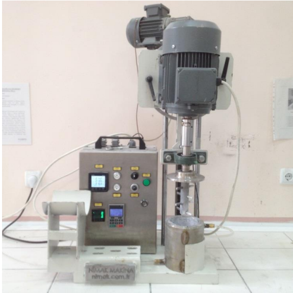
Figure 6. Dry vertical stirred ball mill.
